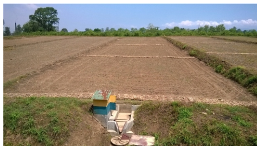
Fig. 3. Layout of agro-geo-textiles (AGT) on 1 m vertical interval or for 100 m long plot, laid AGT after every 25 m length
