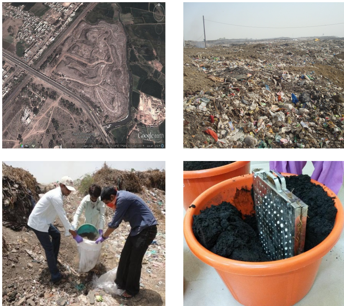
Plate 1. The MSW contaminated site (a, b and c) and strategies to remove heavy metal using customized biofilter harboring fungi (d).
